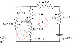
volt battery. This is opposite what battery usually do (they are designed to put energy into the system). As such, the battery in this case can be thought of as depleting energy, suggests a negative power rating.
