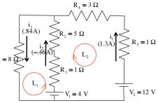
happened to the approximately 220 joules of "left-over" energy provided by that battery? It went into charging up battery  $V_2$  to the tune of -222 joules (this is the approximate overlay—the disparity is due to round-off error).
